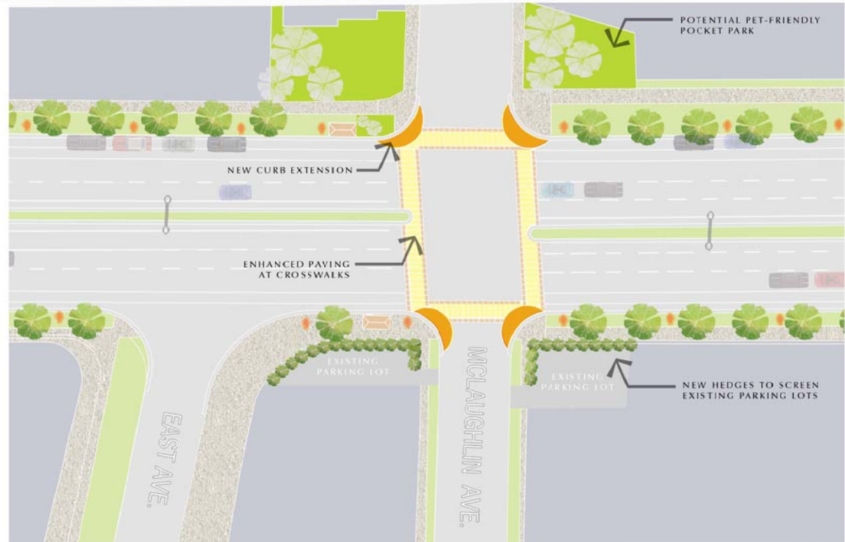
PROPOSED CORNER CURB EXTENSIONS along Venice Boulevard create a safer crossing for pedestrians by reducing the length of the crosswalk. Enhanced crosswalk paving at these intersections clearly mark the major pedestrian circulation paths.
